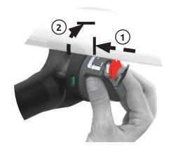
Press and hold the knob while turning the knob towards the car until the signal colour changes to red.
