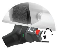
After use, insert the key and turn the key to unlock the tow ball.
