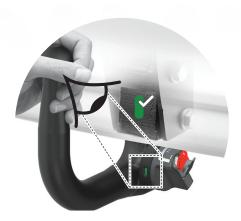
Check if the signal colour is green. Green means a successful lock.
